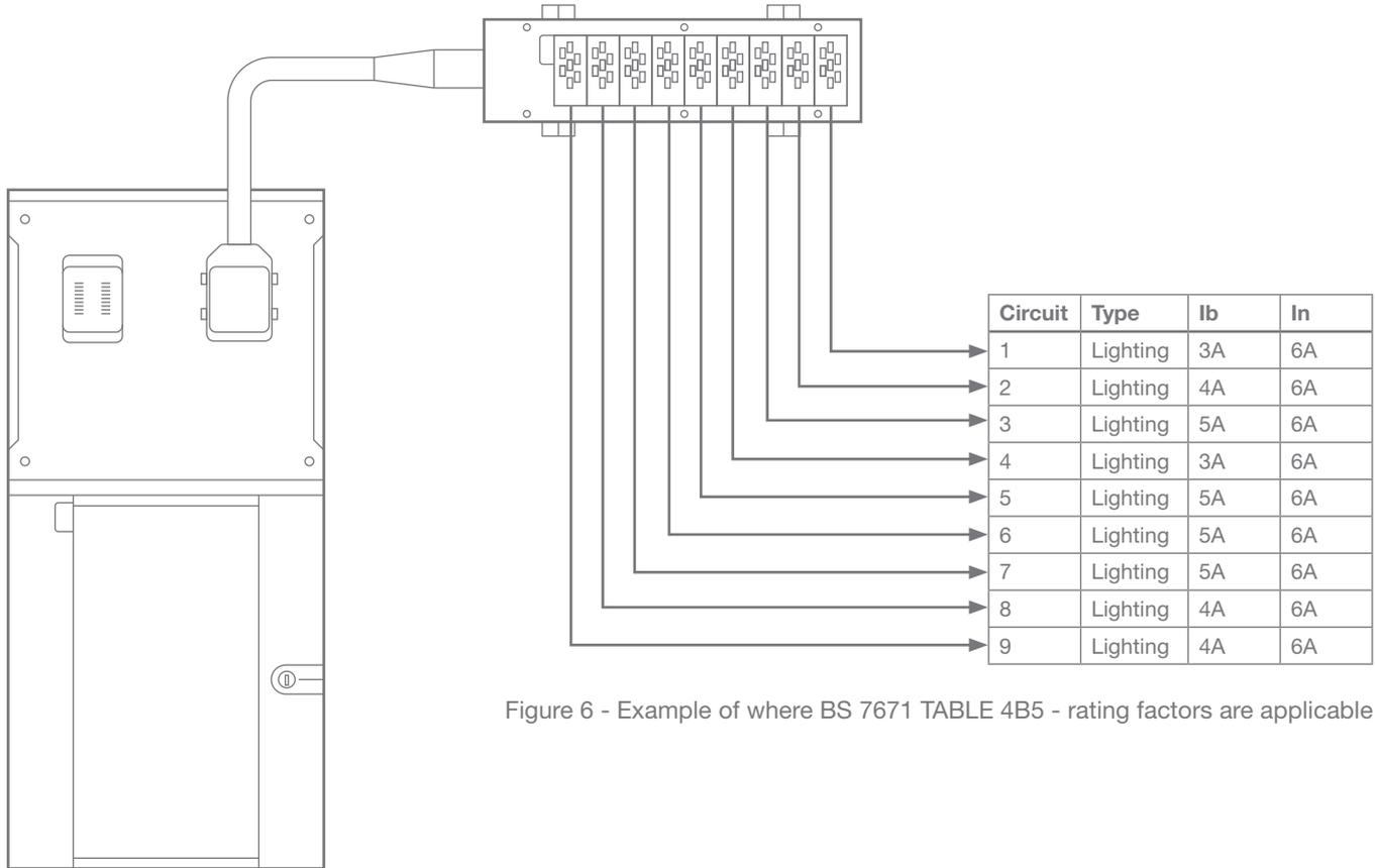
Figure 6 - Example of where BS 7671 TABLE 4B5 - rating factors are applicable
