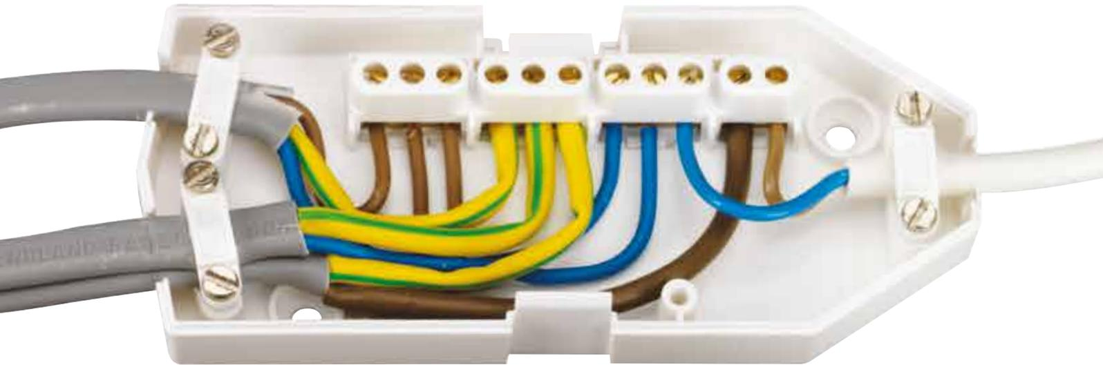
Regulation 526.2 is complied with where the method of connection shall take account of the number and shape of wires forming the conductor. In this junction box solid conductors and flexible conductors can be terminated separately by means of the unique three plate style terminal arrangement.
